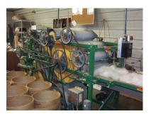
used in quilts and felt making or the web can be consolidated into roving which are further processed into yarns. Blending of colours and types of fibre can be done at this stage.
